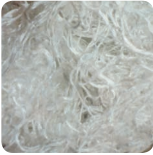
Nylon filament fiber can be produced as microfiber and manipulated to resemble cotton fiber. Its quick-drying characteristic has made nylon a favorite fiber to blend with cotton for lightweight outdoor clothing.
