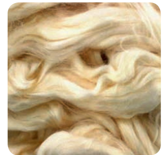
These manufactured filament fibers can look very different from each other due to their fiber shape and the method of cooling the fibers after extrusion from the spinneret. TOP: soy. BOTTOM: bamboo rayon.
